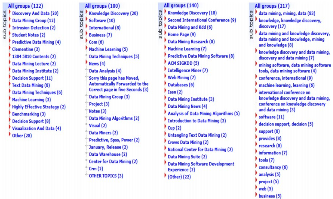
Fig. 5. Comparison of results for a query “data mining” produced by different algorithm (from left to right): TRC, LINGO, AHC and STC. All output were produced using Carrot 2 visualization component.
