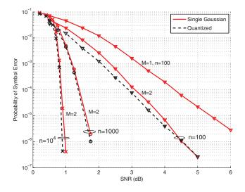
Fig. 2. Probability of symbol error for the single-Gaussian decoder and the quantized-message decoder. The Gaussians mixture size used internally at the variable node is M, and the lattice dimension is n.
