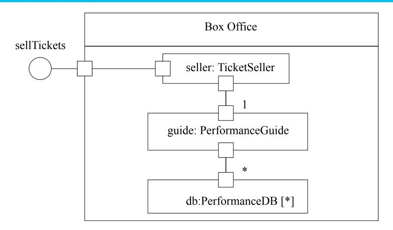
• Each port has a set of provides interfaces and required interfaces that define its external interactions. A provided interface specifies the services that a message to the port may request. A required interface specifies the services that a message from the port may require from the external environment<sub>JAIST Koichiro Ochimizu</sub>
