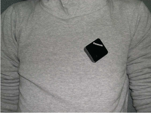
Fig. 1. Mobile c-tag prototype worn by a pedestrian.
