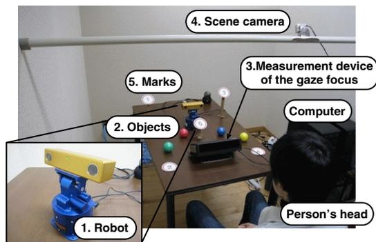
Fig. 2. An experimental environment of human-robot interaction. A person sits in front of the robot(1), and looks at the four rubber balls(2). The measurement device of the gaze focus(3), a scene camera(4), and marks(5) for calibration are located in front of the person.
