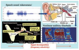
Fig. I Signal representation via auditory filterbank
