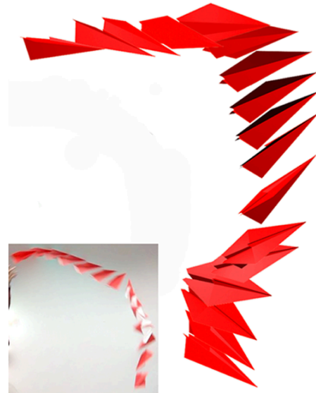
Figure 1: A gliding paper airplane simulated by our stochastic modeling approach. The left-bottom subfigure is a contrastive trajectory captured from a video.
