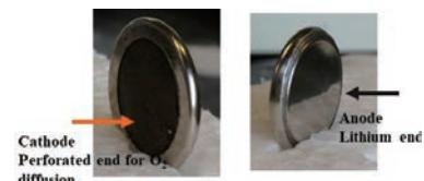
Coin cell configuration of Li-Air Battery
