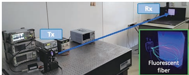
Our recent OWC transmission testbed utilizes fluorescent fiber concentrations at the receiver.
