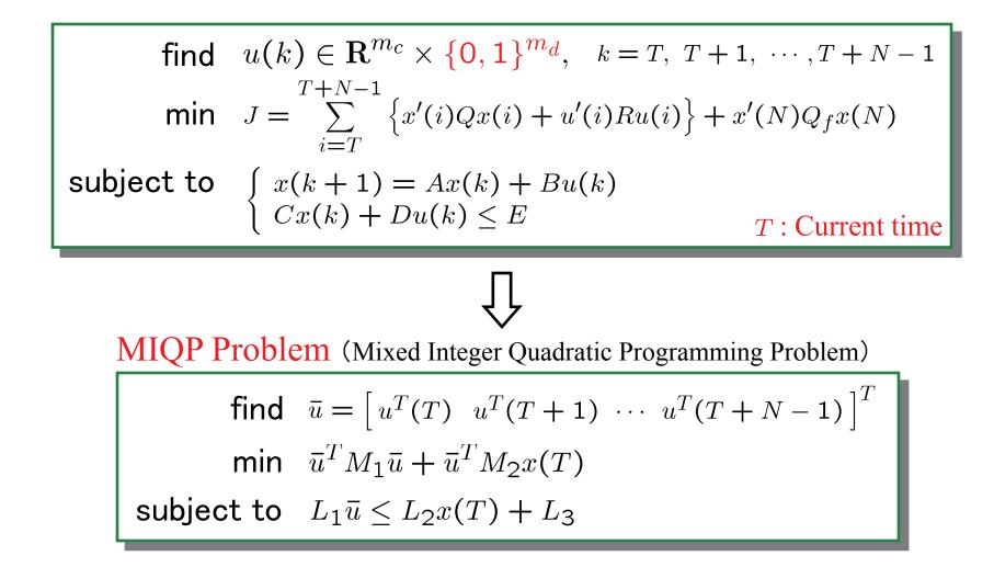
The dim. of continuous variables: $m_c N$ The computation time is too longThe dim. of binary variables: $m_d N$ for practical plants.
