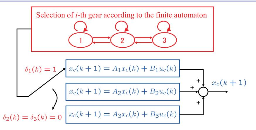
Binary variables  $\delta_1$ ,  $\delta_2$ ,  $\delta_3$  are used.  $\begin{cases} \delta_i(k) = 1 & \text{if Gear } i \\ \delta_i(k) = 0 & \text{otherwise} \end{cases}$   $\implies x_c(k+1) = \sum_{i=1}^3 \delta_i(k) \left( A_i x_c(k) + B_i u_c(k) \right)$  + Model of the finite automaton
