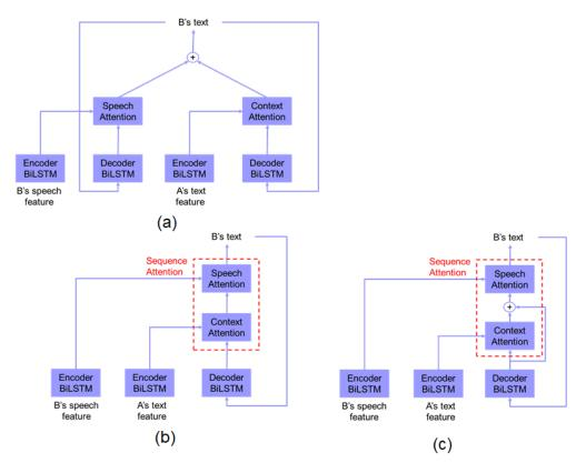
**Fig. 1**. A model of related works: (a) Flat attention combination ("FlatAttComb"); Proposed Models: (b) Sequential attention combination ("SeqAttComb"); (c) Sequential attention combination and bypass connection ("SeqAttComb+Bypass").
