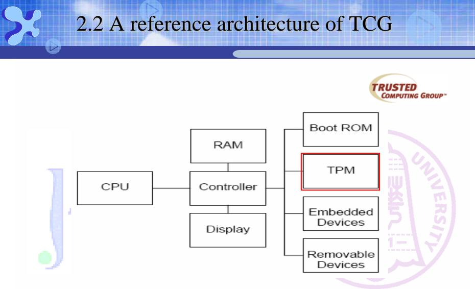
Reference PC Platform Containing a TCG Trusted Platform Module (TPM)
