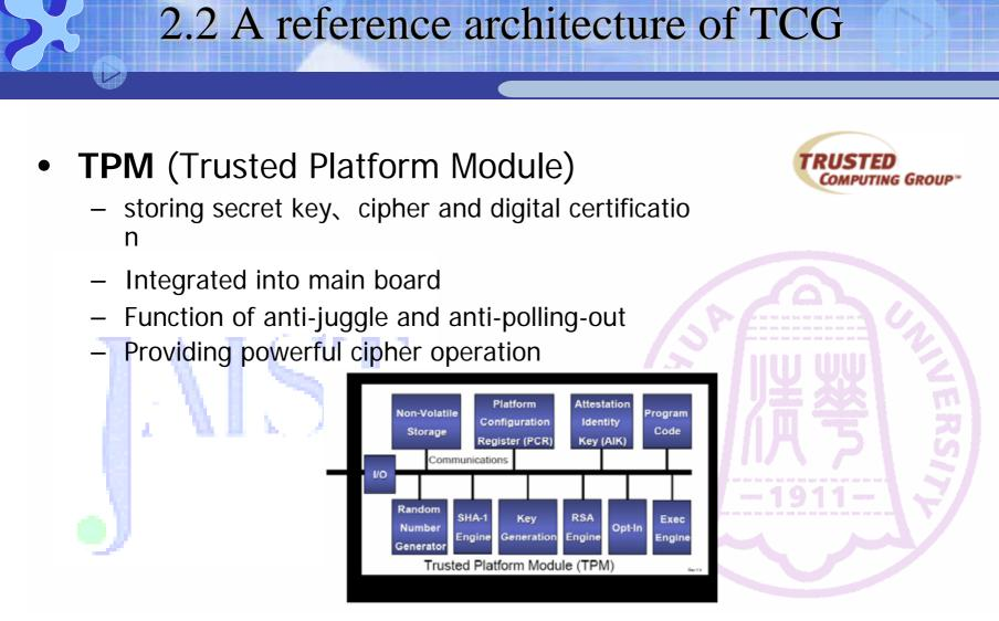
Fig. TPM components architecture
