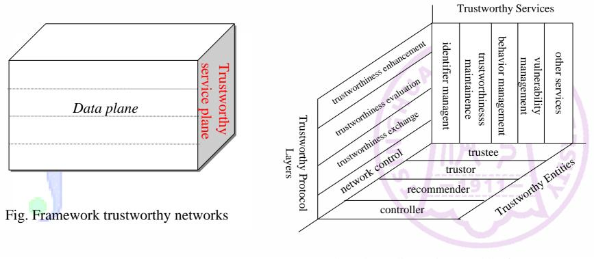
Fig. Three dimension model of Trustworthy Service Plane
