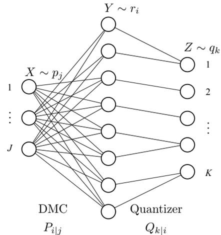
Fig. 1. A discrete memoryless channel followed by a quantizer. Given  $p_j$ ,  $P_{i|j}$  and  $K$ , find  $Q_{k|i}$  which maximizes  $I(X; Z)$ .
