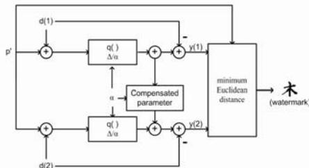
Figure 5. DC-DM QIM detection
