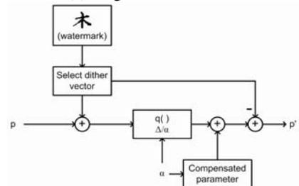
Figure 3. DC-DM QIM quantization.
