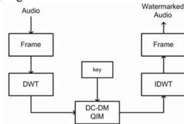
Figure 2. Embedding block diagram.
