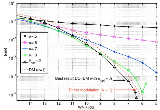
**Figure 2. Performance of uncoded DM and uncoded DC-DM schemes with different  $\alpha$ .**
