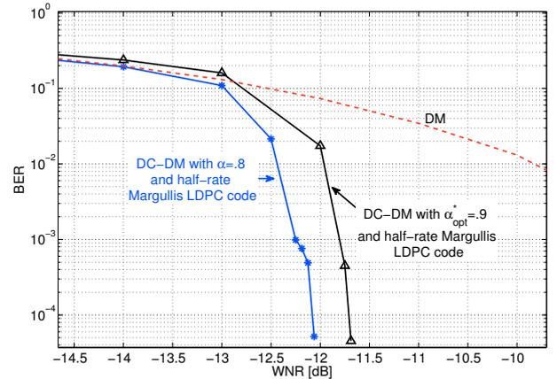
**Figure 3. Performance of DM and DC-DM with  $\alpha$  lower than theoretically optimal.**
