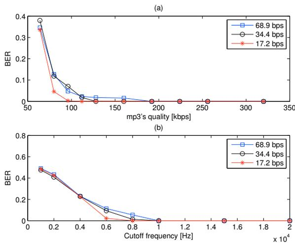
**Figure 5. Watermark robustness against: (a) MP3 and (b) low-pass filtering.**
