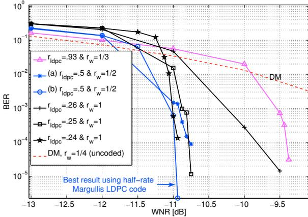
**Figure 1. Performance of DM with LDPC codes and uncoded DM.**
