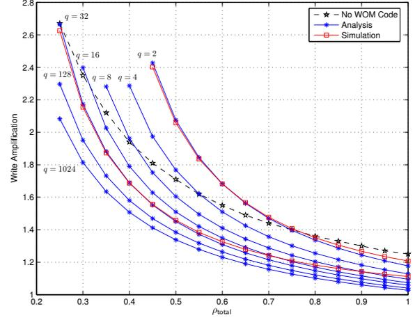
Fig. 2: Simulation results for different  $q$  when  $t=2$ .
