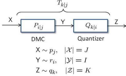
Fig. 1: A discrete memoryless channel followed by a quantizer. Given  $p_j$ ,  $P_{i|j}$ ,  $0 \leq \rho \leq 1$ , and  $K$ , find  $Q_{k|i}$  which maximizes  $\tilde{E}_0(\rho; Q)$ .
