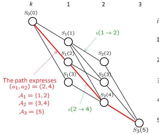
Fig. 3: Trellis-type illustration showing the relationship between state metrics for  $I = 5$  and  $K = 3$ .
