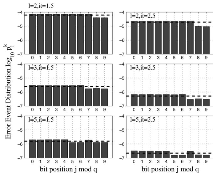
Fig. 2. For the unequal error protection code, error event distribution  $p_1^k$  versus beginning bit position  $k = j \bmod q$ , for event lengths  $l = 2, 3, 5$ , after 1.5 and 2.5 turbo iterations, at an SNR of 9 dB. Dashed lines show the error event distribution for the single-parity check code.
