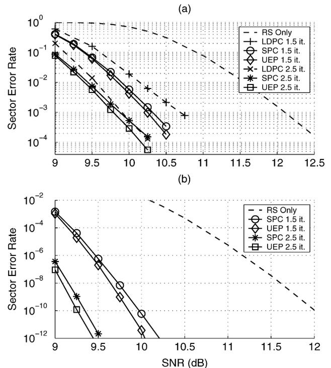
Fig. 3 (a) SER simulation of single-parity check (SPC) codes,  $r = 2$  unequal error protection (UEP) codes, and  $j = 2$  LDPC code; assuming a  $t = 3$  RS code. (b) SER analysis for SPC and UEP codes, assuming a  $t = 10$  RS code.
