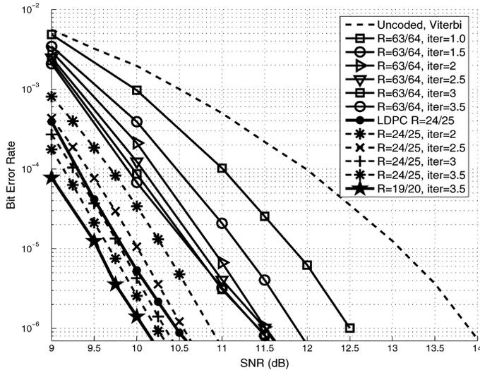
Fig. 1. BER of interleaved single-parity check codes for various rates; a column weight 2 LDPC code, decoded for 3.5 iterations, is shown for reference.
