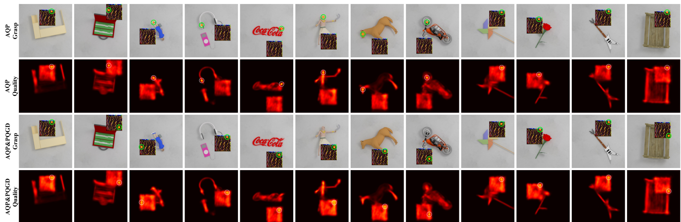
Fig. 6. The meaning of each row is consistent with Fig. 5. Here, the SE-ResUNet and the Jacquard Grasp dataset are used to optimize the AQP. And AQP is scaled to 0.3 of the original size (the same size as the image).
