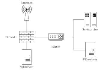
Figure 8. Network topology for the experiment scenario.
