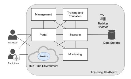
Figure 1: Generic architecture for a full-fledged cybersecurity training platform.
