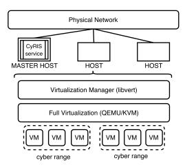
Figure 4: The architecture of the system running CyRIS.
