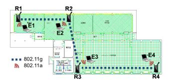
Figure 2: Wireless router deployment: the physical realm of our prototype hybrid experiment platform.
