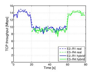
Figure 5: TCP throughput results versus time for experiments with multiple senders.
