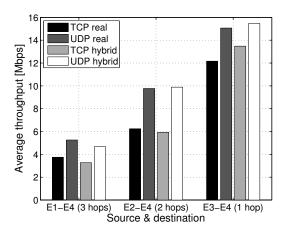
Figure 4: Average throughput results for experiments with single senders.
