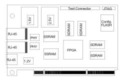
Fig. 1. Floor plan of the PCI card.
