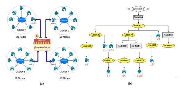
Figure 4. (a) The network model and (b) the power grid model of IEEE 13 node test feeder with 73 Houses.
