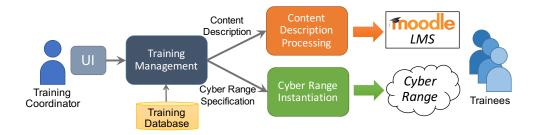
Figure 3: Architecture of the CyTrONE cybersecurity training framework.
