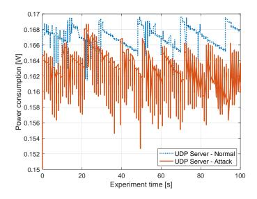
Figure 9: UDP server power consumption for the normal and flooding attack scenarios.
