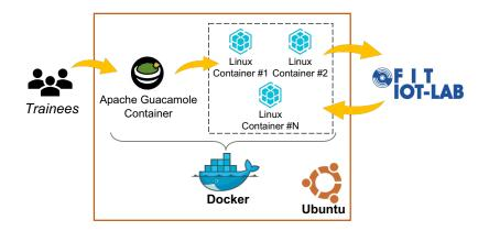
Figure 7: Overview of the IoTrain-Lab architecture.
