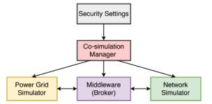
Fig. 3: General architecture of the co-simulation approach for smart grid cybersecurity experimentation
