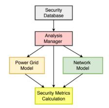
Fig. 4: General architecture of the analytical modeling approach for smart grid cybersecurity experimentation
