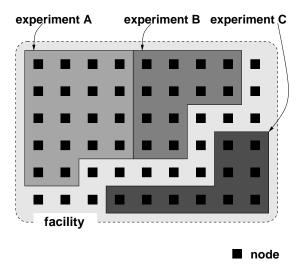
Fig. 2. Using space division of the facility
