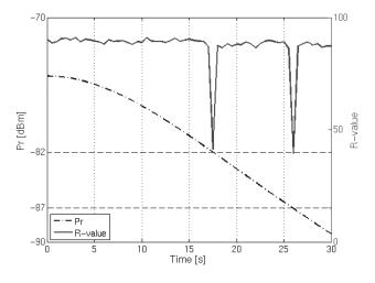
Figure 4: Received signal power, *Pr*, and the E-model output, R-value, versus time
