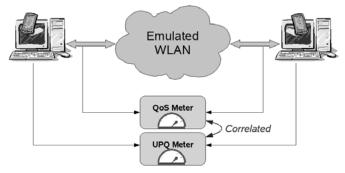
Figure 3: WLAN emulation for application performance assessment
