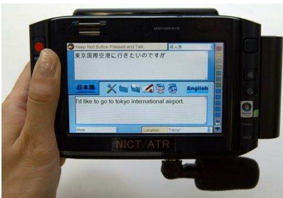
Figure 6. A hand-held terminal device of the NICT/ATR multilingual speech-to-speech translation system.
